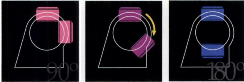
Detectors move from 90° for cardiac SPECT to 180° for total body and general SPECT imaging at the touch of a button.
