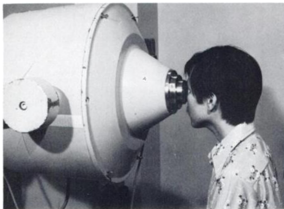
FIG. 1. Position of patient for nuclear dacryocystography. (A) Collimator base; (B) pinhole insert.
