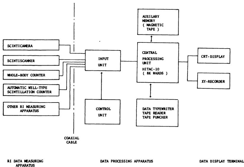
**FIG. 1.** Block diagram of radioactive isotope data-processing system.
