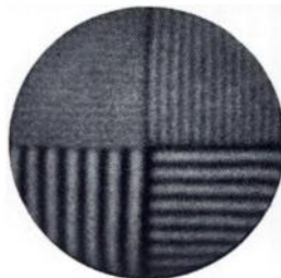
OVERALL RESOLUTION 99mTc, 999 K-counts, Window:20% Collimator: Super High Resolution, Phantom to Collimator distance:10cm
