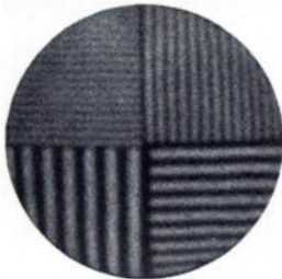
INTRINSIC RESOLUTION 99mTc, 999 K-counts, Window 20%
